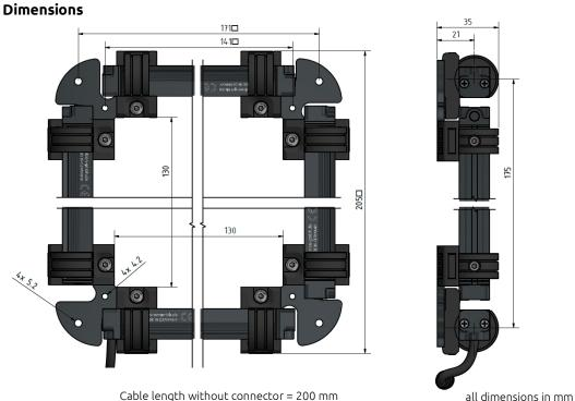
Cable length without connector = 200 mm
